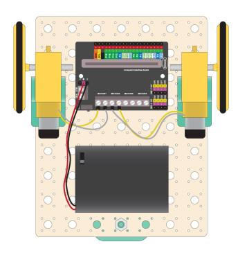
For the remote control you will need another Microbit. So you will have two microbits, one in the controller and one in the robot. We will use the radio feature of the Microbit to send messages from the controller to the robot:
