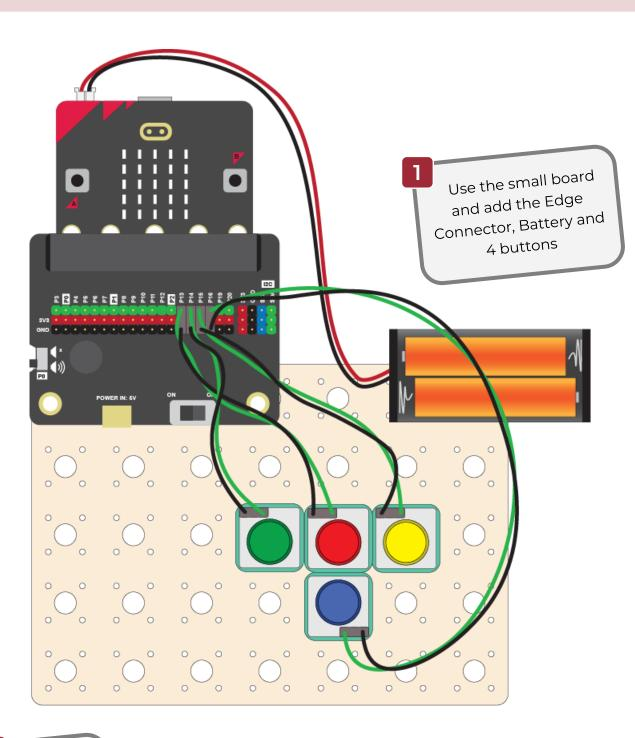
Wire up the buttons as follows using GS wires
